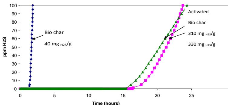
Figure 1 H<sub>2</sub>S Absorption from a 400 ppm gas stream
