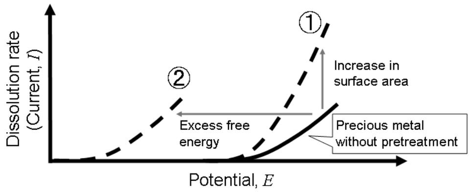
Figure 1 Two explanations for enhanced dissolution of precious metals by alloying.
