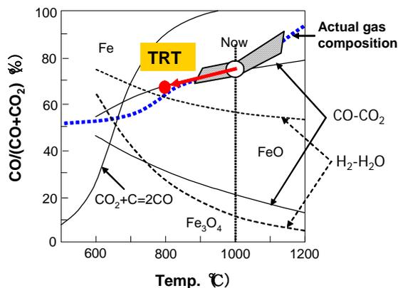
Fig.1 Fe-FeO-CO-CO<sub>2</sub> equilibrium in the blast furnace.
