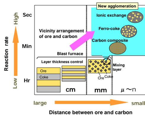
Fig.2 Acceleration of reaction rate by vicinity arrangement of ore and coke.
